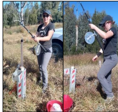
Sampling methods: bailer (left) and net sampling (right) for collection of stygofauna (Photo: G Hose 2022)
