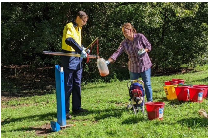
Figure 30. Field sampling demonstration at Macquarie University, where bailer (shown here), net and pumping methods for collecting water, stygofauna and eDNA were explained to workshop participants
